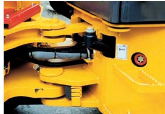
Articulation/swivel joint with ELGES spherical plain bearings
