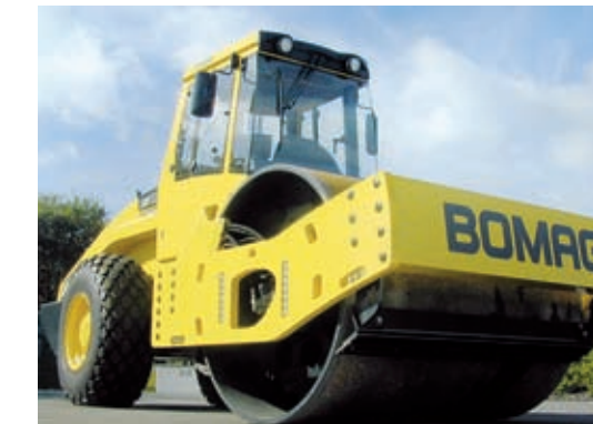
Vibratory roller with four-point contact ball bearing and maintenance-free ELGES spherical plain bearings in articulation/swivel joints (photo: BOMAG)
