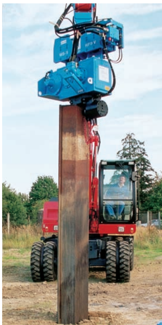
Dynamics required: Cylindrical roller bearings LSL can withstand high accelerations - important e.g. for vibrators in vibratory compaction equipment (photo: ThyssenKrupp)
