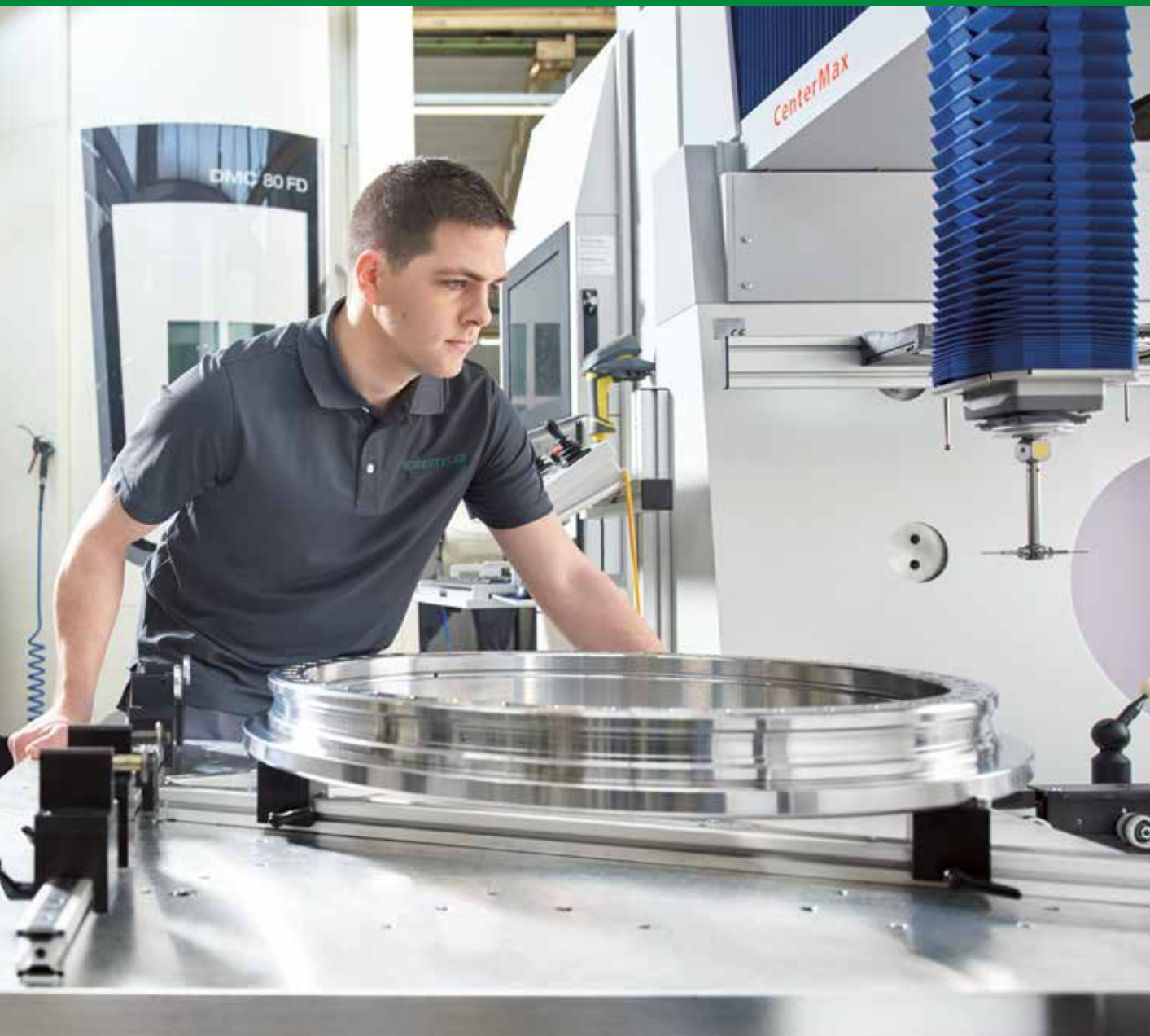
Top Michael Sperber operating the 3D measurement machine, whose measurement data is transmitted back to the Machine Tool 4.0 for analytic purposes.
