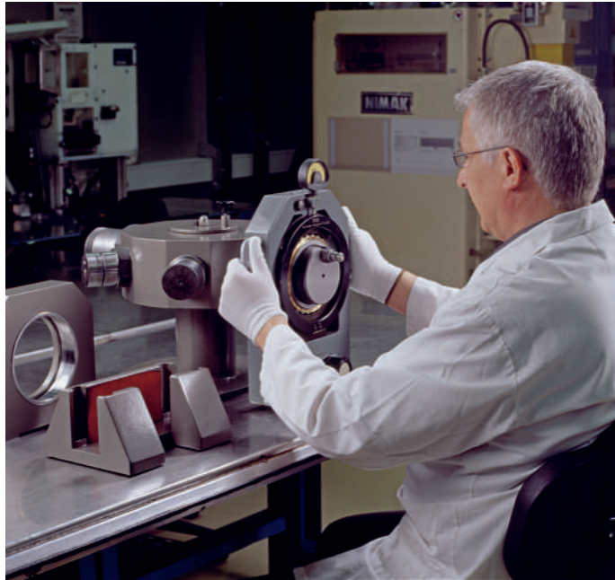
34 Positioning the enveloping circle gauge
