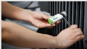
**Plug :** The vibration sensors are attached to each machine using screws or adhesive. Then they are activated via NFC.
