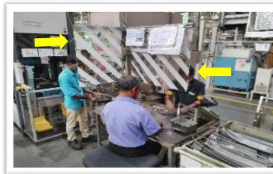
Side Protection at Sub Assembly and Station with Acrylic Sheets
